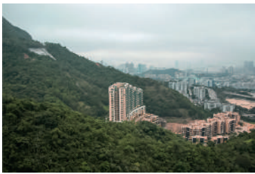
2 The possibility of the city to grow is constrained by the limited area of flat land: Since the gradient of most of the slopes is more than 1:3 and the soil is of very loose consistency, the city develops only on the scarce flat land at the foot of the hills.
