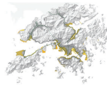
14 Public transportation network and reclaimed land in Hong Kong: Land reclamation was introduced for the first time in the 1890s. Today 12 percent of Hong Kong's urban area is located on reclaimed land, virtually all of which is connected to the public transportation network.
